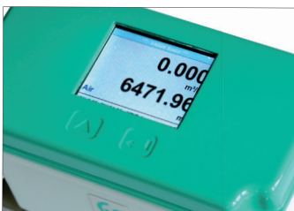
Flow measuring ranges VA 525 (max version 185 m/s) for compressed air (ISO 1217:1000 mbar, 20 °C) Measuring ranges for other types of gas see pages 114 to 117
