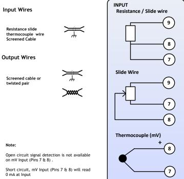
CONNECTION For cable length < 3 Metres no screen or twist pair required. Use recommended types for cable length (3 to 30) metres.
